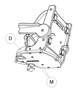
Both cushions can be attached to the chair by aligning the holes in the cushions with the corresponding holes in the frame. Then two bolts per cushion need to be inserted through the frame and threaded into the inserts that are in the cushions.
