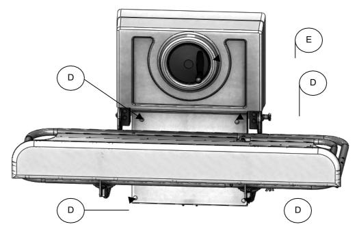
• Fit the hand wheel (E) to the spindle and secure in place with a M8 x 16, and 1 x M8 flat washer. Operate the hand wheel to ensure the shower stretcher raises and lowers satisfactorily. Press in place the plastic dust cap.
