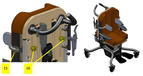
If ordered, the laterals will come attached to the chair however they can easily be removed and attached if necessary. The **height** and **width** of the laterals can be adjusted and each lateral can be **swung away** from the chair for ease of access.
