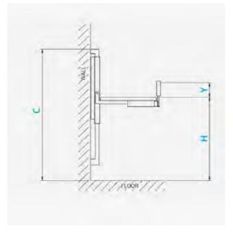
The diagram above shows the relevant dimensional sizes of the Changing Bench. Below *(Table 3)* is a table containing the dimensions of each size. All dimensions are in mm unless otherwise specified.
